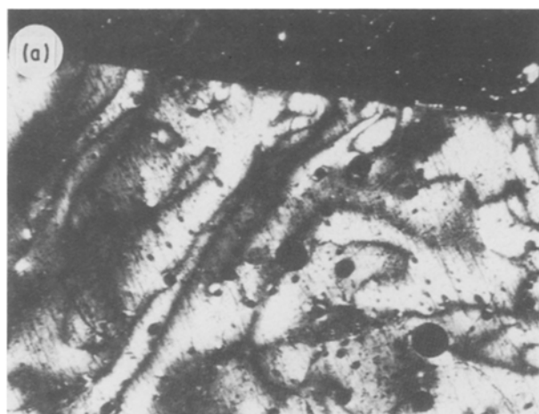
Figure 3 Optical photomicrographs of blends of MP-A with PVCP-1. Amount of blended PVCP-1: (a) 10 wt %, (b) 20 wt %, (c) 30 wt %.
